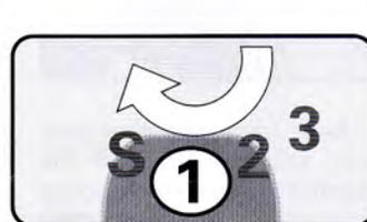
7. The film counter will count the no. of picture you have already taken. The counter will automatically return to 'S' when open the film door.
