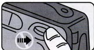
1. When you have reached the end of film, the film advance wheel will stop. **DO NOT OPEN THE FILM DOOR YET !** You must rewind the film first.
