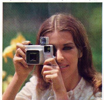
he Autopak 500 calculates whether or not you have to use flash. All you have to do is attach the flashcube, focus, then press the shutter release. When your first flash photo is taken, the flashcube rotates automatically to the next bulb ... and you're ready to shoot again. You can attach a flashcube to your Autopak 500 even when you're photographing in bright daylight. But don't worry about the flash going off. If your light is sufficient and flash is unnecessary, the flashcube does not go off.
