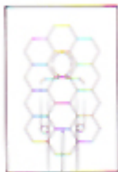
No matter where your subject appears, honeycomb-pattern metering precisely measures exposure levels in 14 separate areas of a photograph.
