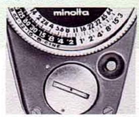
Simply press a red test button and the indicator lock button simultaneously to check the condition of the single mercury battery at a glance. The needle will swing to a red spot on either the high or low light intensity scale to show good battery condition. The case of the Viewmeter 9 is made of extremely durable polycarbonate material—tough enough to withstand all the rigors of hard professional use.
