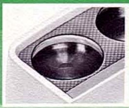
The CdS cell on the Minolta Viewmeter 9 will accurately measure anything from candlelight to bright outdoors. Precise readings are possible even in moonlight. An exclusive blue filter over the CdS cell automatically compensates for changes in color temperature, permitting extremely accurate measurement for exposure of color film.
