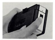
Slide the back cover release button up; the cover opens automatically.
