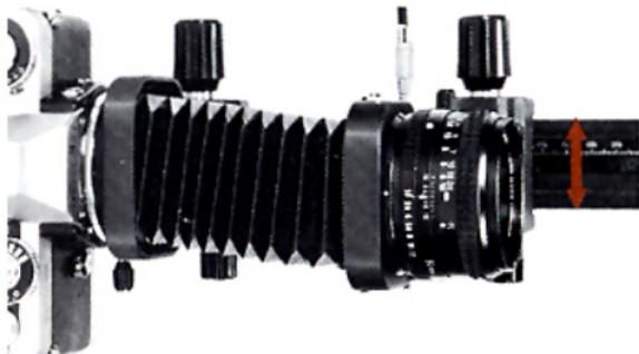
When photographing subjects positioned diagonally with the film plane, you may find that depth of field, even at smallest apertures, will not make important subject points acceptable sharp. At these times, swinging the lens standard towards the principle plane of the subject will help to improve the over-all sharpness of the image.
