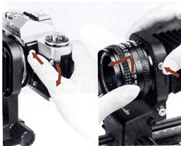
While pushing the lens-release button of either the camera or bellows, turn the lens or camera body counterclockwise as far as it will go and lift it away from the bellows.
