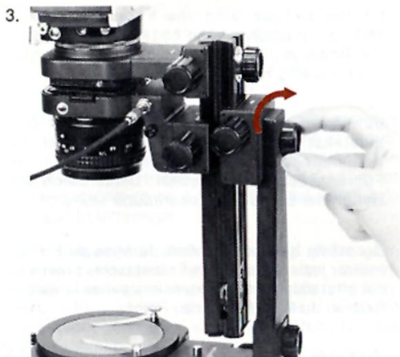
Secure the focusing rail to the Macro Stand or a tripod by means of the socket provided. To focus, unclamp the Focusing Rail and turn the focusing knob until the subject appears sharpest in the viewfinder. Then clamp the rail.
