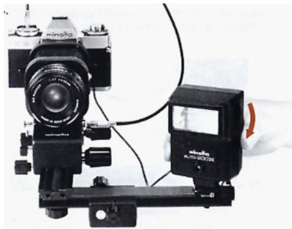
After setting bellows extension and focusing, turn the flash so that it points directly towards the center of the subject and measure the flash-to-subject distance.
