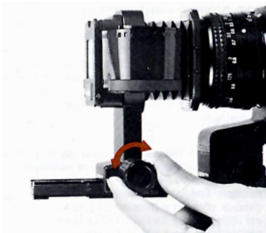
Consult the magnification tables to find the amount of extension necessary for the lens in use and the magnification desired and adjust and clamp the bellows. Then focus by turning the focusing knob on the copier's standard.
