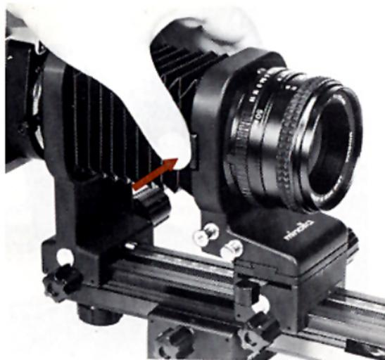
Depress the tabs on both sides of the lens standard and detach the bellows.
