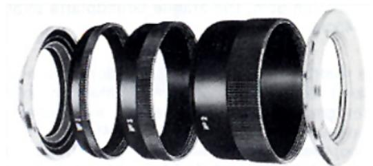
This set of five separate tubes can be used in various combinations for close-up photography with Minolta lenses. Function of the tubes is to increase magnification by lengthening the lens-to-film distance. Selection of the proper extension tube or combination depends on the area to be covered or the image size required. When used with TTL Minolta SLR cameras, no compensation for exposure is necessary since exposure readings may be taken directly through the tube and lens combination.
