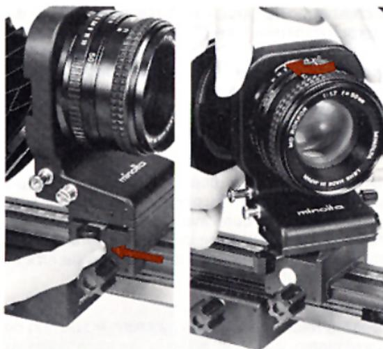
Slide the swing-clamp lever towards the camera and rotate the lens standard on its pivot until the front of the lens faces the camera (a detent will hold it in position). Slide the lever away from the camera to lock the lens standard in place.
