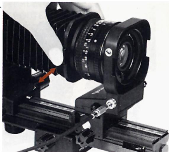
While depressing the tabs on both sides of the frame, insert the raised circular lip of the bellows' frame into the threaded filter ring in the front of the lens.
