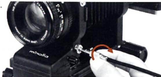
Screw the end with the engraved red ring into the socket on the side of the lens standard opposite the stop-down/shutter-release button.
