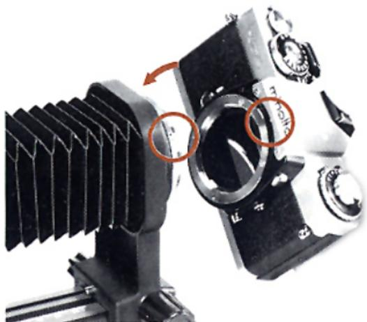
Align the red indexes on the camera and bellows, insert the bayonet into the socket and turn the camera body clockwise until it locks in place with a click.
