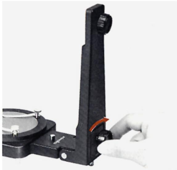
Unfold the Macro Stand's support column and secure it with the fixing screw.
