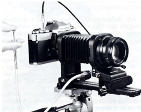
Release the shutter, making sure to keep the stop-down/shutter-release or cable-release button pushed all the way in until the exposure is complete and the shutter has closed. For best results, use the Minolta Cable Release II in its pre-locked position.
