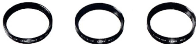
These lenses screw into the filter mount of normal lenses to permit focusing at close-up distances. Lenses 1 and 2 may be used in combination to allow work as close as 23cm (9 in.) from the subject. Lens 0 allows closer focusing with short telephoto lenses. With any of these close-up lenses, aperture is set as it would be for normal photography.
