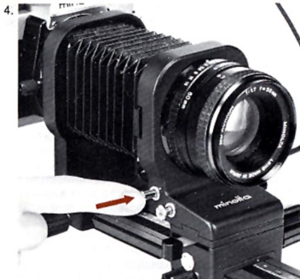
With the shutter cocked, depress the stop-down/shutter-release button. If the shutter releases, no adjustment is necessary. If it does not, keep the button pushed all the way in and turn the adjustment collar until the shutter releases.
