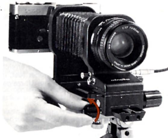
Loosen the clamps on the camera and lens standards by turning them counterclockwise. Then turn the control knob on either standard to set the bellows extension as indicated in the close-up tables for the lens in use and magnification desired.
