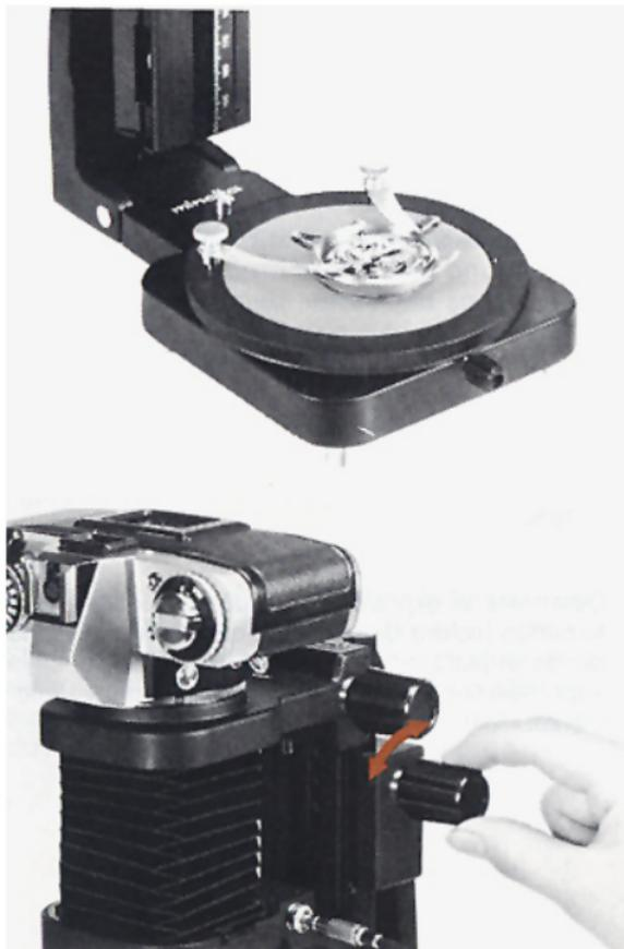
5. Determine exposure after the lighting is set by taking meter reading of the reflected light from the Macro Stand's gray insert plate whose surface has standard reflectance of 18-percent.
