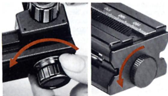
While the bellows-focusing rail assembly mounted on a tripod, loosen the Focusing Rail's attaching screw about a quarter turn and remove the connecting plate.
