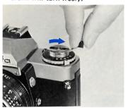
When you are certain that the film is completely rewound, pull the back-cover release knob to open the back and remove the cartridge.
