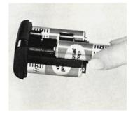
Insert the battery holder into the winder body so that the white marks are on the same side and snap it securely into place.
