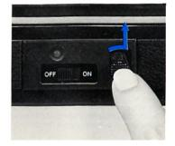
3. Fold out the rewind crank and turn it in the direction indicated by the arrow on it until the red Safe Load Signal bar moves out of the window to the left. You will then feel tension on the film increase and disappear, and the crank will turn freely.
