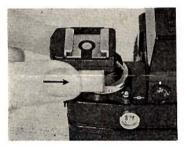
To install the accessory hot shoe, slide it onto the accessory mount located at the bace of the backcover release knob on the camera body. It will lock in place automatically.
