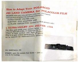
Kit of accessories adapts the J33 to use Type 48 color film. This adapts the exposure system for the far slower speed of the color film (ASA 75 rather than 3000).
