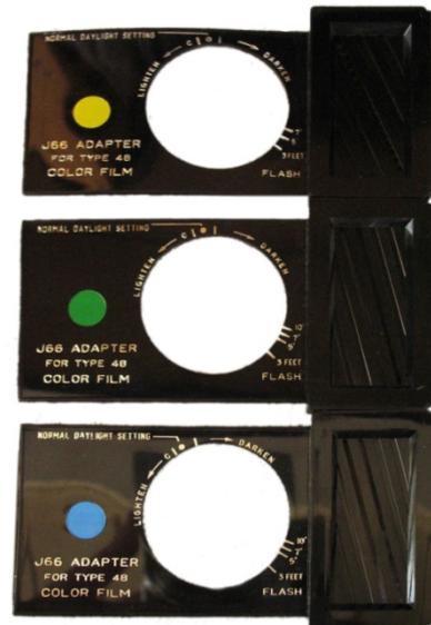
Kit of accessories adapts the J66 to use Type 48 color film. The kit includes three clip-on front plates (#566) which block part of the selenium cell and provide new calibration marks for the lighten/darken control - this adapts the exposure system for the far slower speed of the color film (ASA 75 rather than 3000).
