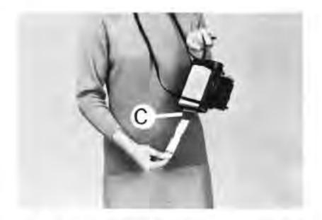
2. Pull the white tab (B) all the way out of the camera: This causes a yellow tab (C) to pop out of a narrow door in the end of the camera. Be sure that the neck strap of the camera does not block the tab slot during tab pulling.
