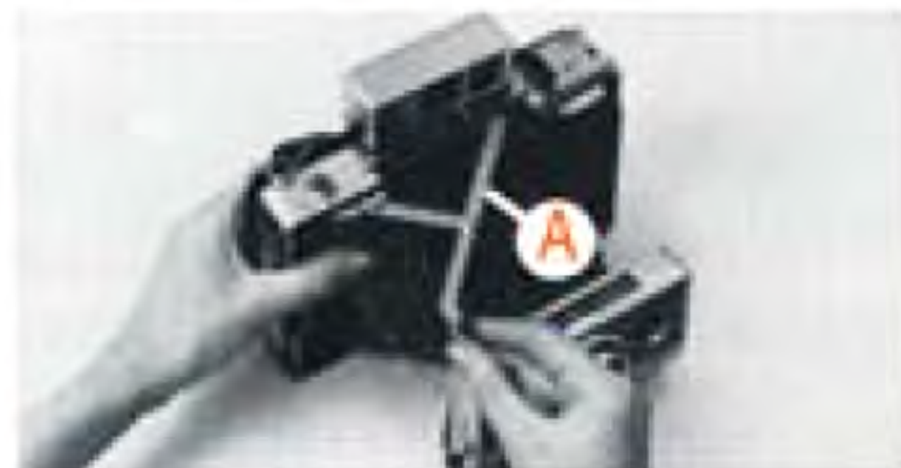
5. Pull camera front out as far as it will go. Be sure locking bar (A) snaps into place. If not, you may get blurred or all-black pictures.
