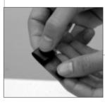
Cut the shield tape about 2 inches (5 cm) and fold back about 1/2 inch (1 cm).
