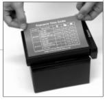
Place the inner box above the film holder. Center the openings.
