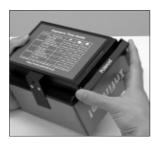
We Hold the top and bottom of film holder latch, and turn it into outside.
