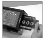
Close the film holder latch. Pull the safety cover out in a straight line in one motion. Do not hold the camera body when pulling out the safety cover or film. Hold the film holder.
