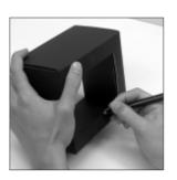
Paint the frame of the inner body box opening with a black marker pen.
