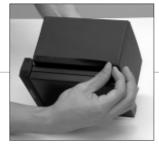
To prevent light seeping into the box, apply the shield tape around the film holder.
