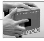
After exposure, cover the pinhole with shield tape.
